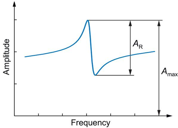
Figure 7: Resonance with parasitic signal component; the maximum amplitude of the resonance behavior is smaller than the maximum of the overall signal.
