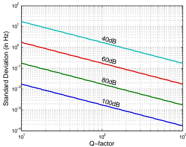
Figure 8: Typical standard deviation of measured resonance frequency for a resonator at 30 kHz as function of  $Q$  and  $\text{SNR}_R$ .
