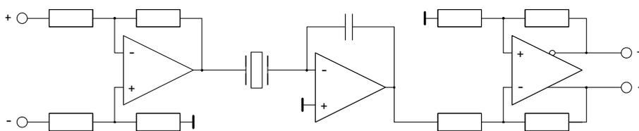
Figure 5: Sensor frontend for a quartz tuning fork resonator (simplified).
