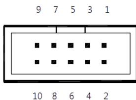
Figure 2: Extension Connector Pin Numbering (Receptacle, Front View)
