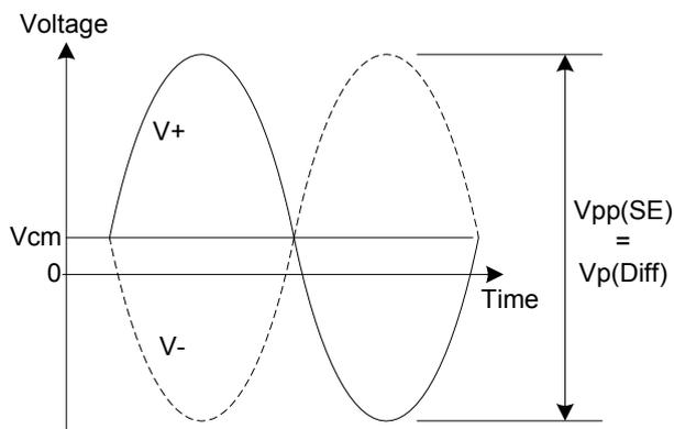
Figure 4: Differential signal levels.
