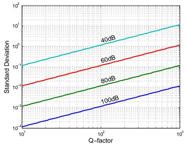
Figure 9: Typical standard deviation of measured quality factor for a resonator at 30 kHz as function of  $Q$  and  $\text{SNR}_R$ .
