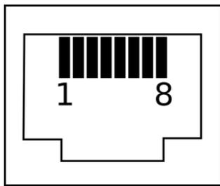
Figure 1: Sensor Port Pin Numbering (Receptacle, Front View)
