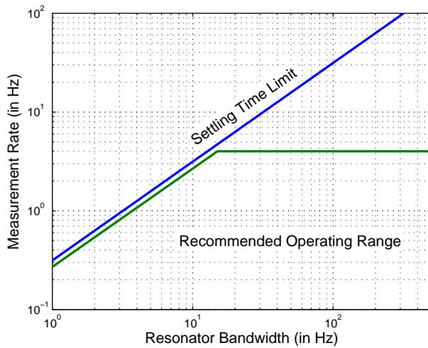
Figure 6: Measurement rate vs. resonator bandwidth.
